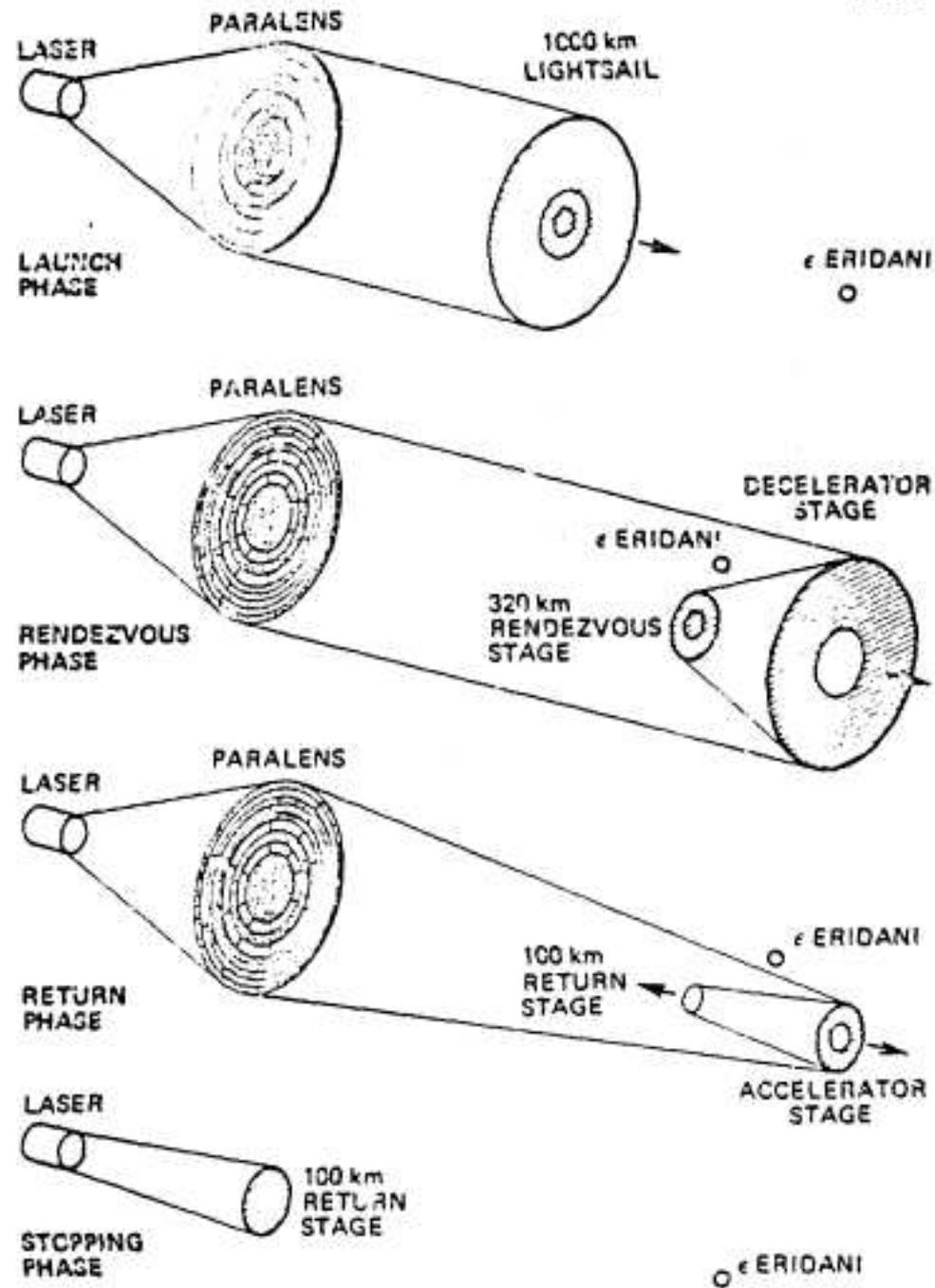
Figure A-2. Roundtrip Interstellar Travel Using Laser-Pushed Lightsails.
